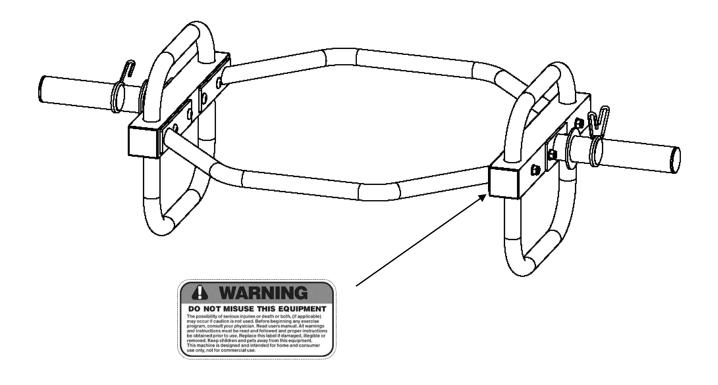
The Warning Label shown here has been placed on the base of Handle Assembly. If the label is missing or illegible, please call customer service at 1-800-999-8899 for replacement. Apply the label in location shown.
