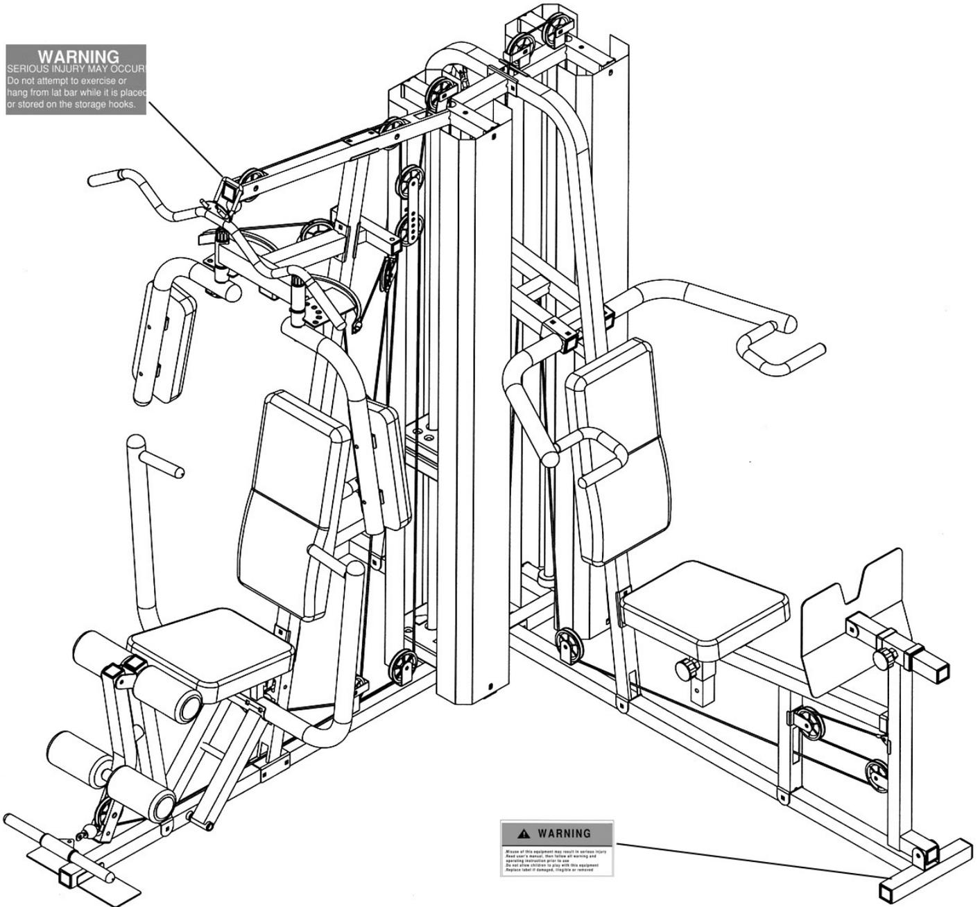
The warning labels shown here have been placed on the Rear Base and Upper Frame. If the labels are missing or illegible, please call customer service at 1-800-888-8899 for replacements. Apply the labels in location shown.
